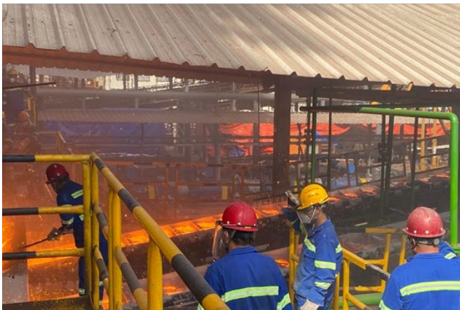
NPI being poured into an Ingot caster
